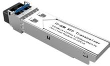
G311SM is single-mode optical fiber module. Support optical fiber transmission to extend LAN area and bandwidth, good to extend the networking coverage in large and middle LAN. Compliant with IEEE802.3z standard and working on 1310nm mode. Small size design and can be built-in switch with small space. Internal power by switch and easy installation, can be matched well with IP-COM series switch which owns SFP port.
